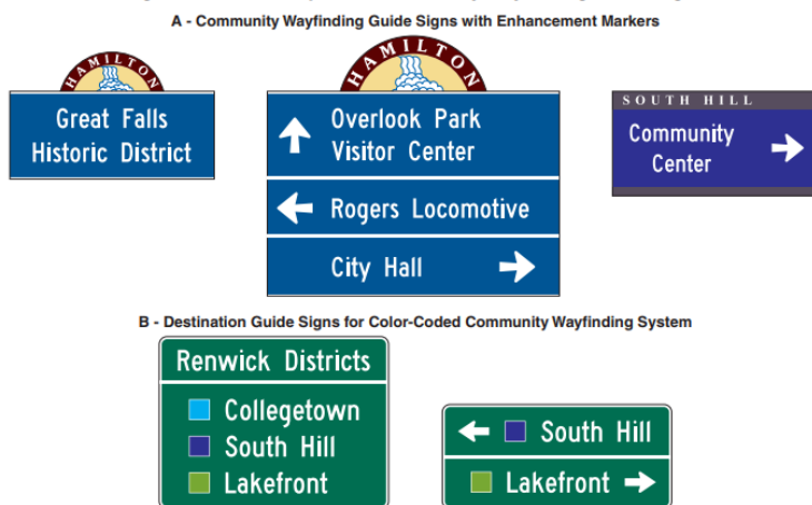
Figure 2D-18. Examples of Community Wayfinding Guide Signs
